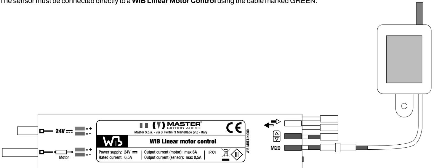
To connect to two control units, the WIB.SMT.004.000 splitter must be used.
