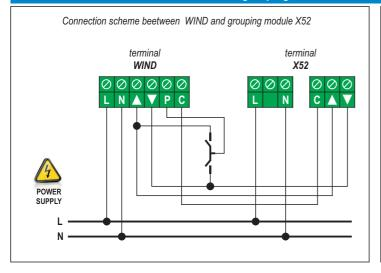
Connection scheme beetween WIND and grouping module X54
