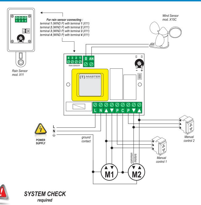
IN ORDER TO CHECK THAT CONNECTIONS HAVE BEEN CARRIED OUT AS IN THE SCHEME, BRING THE AWNING TO THE INTERMEDIATE POSITION AND ROTATE THE SENSOR BLADES SINCE WIND ALARM BEGINS. THE AWNING MUST MOVE UPWARD. IF THE AWNING MOVES DOWNWARD REVERSE THE OPERATION WIRES OF MOTOR OR MOTORS.
