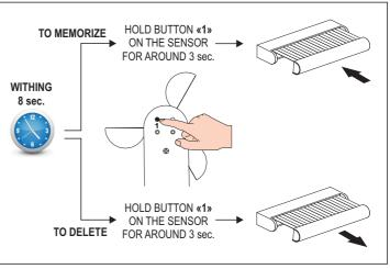
IF THE RECEIVING DEVICE IS SWITCHED ON AFTER A TEMPORARILY ABSENCE OF POWER SUPPLY, IT TAKES UNTIL 10 MINUTES TO RE-ESTABLISH THE RADIO TUNING WITH THE RADIO SENSOR.
