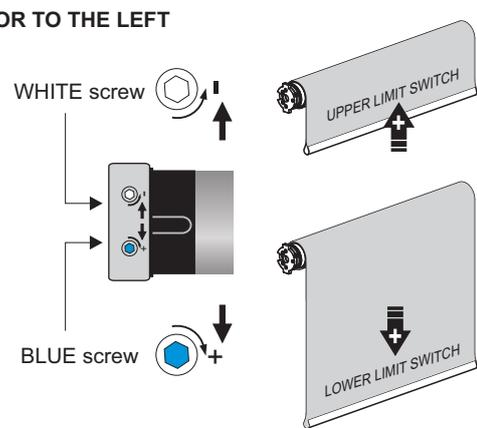
If the fabric is wrapped from behind the roller: the blue screw adjusts the lower limit switch, the white screw adjusts the upper limit switch
