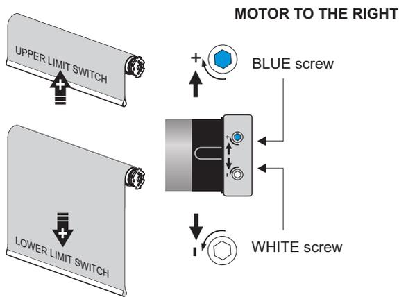
If the fabric is wrapped from behind the roller: the blue screw adjusts the lower limit switch, the white screw adjusts the upper limit switch
